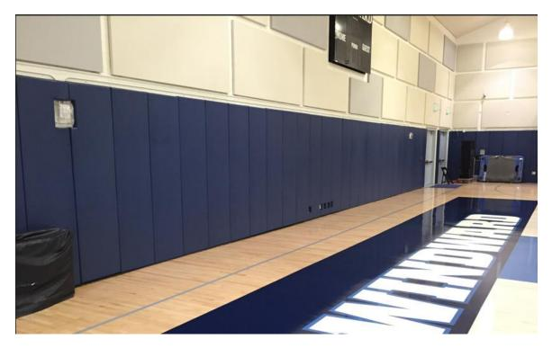
Standard gymnasium wall padding is constructed with 2" Polyurethane foam, which is mounted on a 7/16" OSB Wood Backing and wrapped in 18 oz Solid Vinyl. Standard finish with 1" nailing lips top and bottom. Pads are custom fabricated to fit wall areas.
